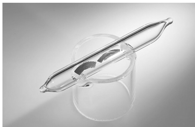
Figure 1. A sample of pure beryllium metal under argon in a sealed ampoule. Picture: A. Heddergott.
